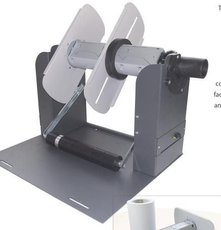
The L801 Series' optional motorized core rewinder is a robust, reliable addition to your L801 Digital Label Printer. It handles labels up to 8.5" wide and can rewind rolls having an outside diameter up to 8.0". Rolls are rewound onto a 3" core.
